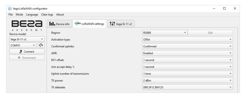
**Region** - allows you to select one of the frequency plans available on the device or set custom frequency plan. The custom frequency plan operates on the basis of the EU-868 frequency plan.
