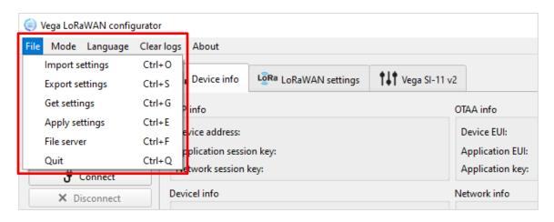
File server — opens a client interface to download firmware, software, drivers, user manuals, and other materials directly within the "Vega LoRaWAN Configurator" application.
