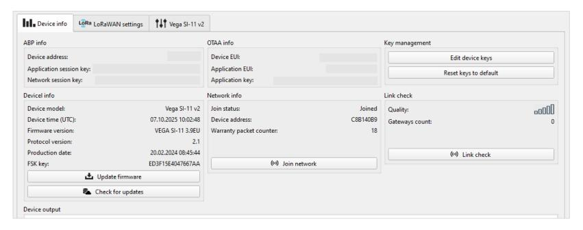
**ABP info** - displays the data necessary to register the device in the LoRaWAN® network with ABP method (Activation By Personalization).
