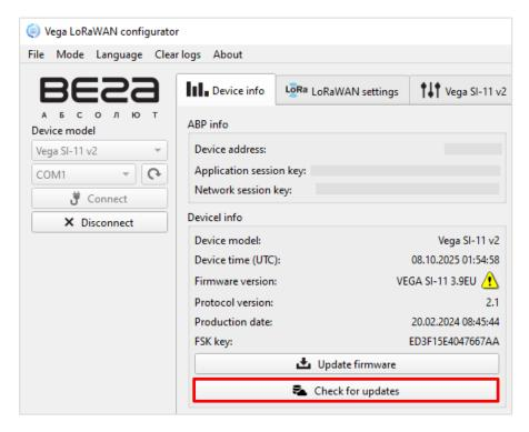
Update firmware - allows you to select the firmware file from your computer's hard drive and load it into the device. The device will automatically disconnect from the configurator when the download is complete. The latest firmware version for the device is available for download on the <a href="iotvega.com">iotvega.com</a> website on the corresponding product page or via the built-in client in the "Vega LoRaWAN Configurator" program on the file server.
